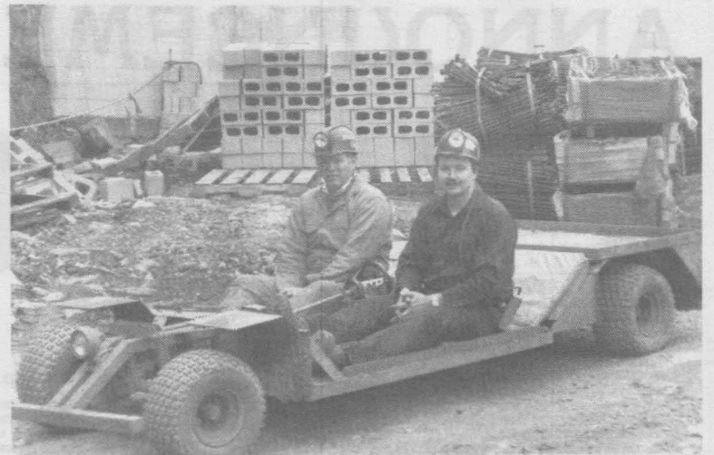
KENTUCKY MINE —Senior Plain Truth writer John Halford (left) and surveyor Mike Stewart sit in a mouse, which can navigate the low mine shafts at the Kiah Creek coal mine in Kentucky. [Photo by Doug Peitz]
